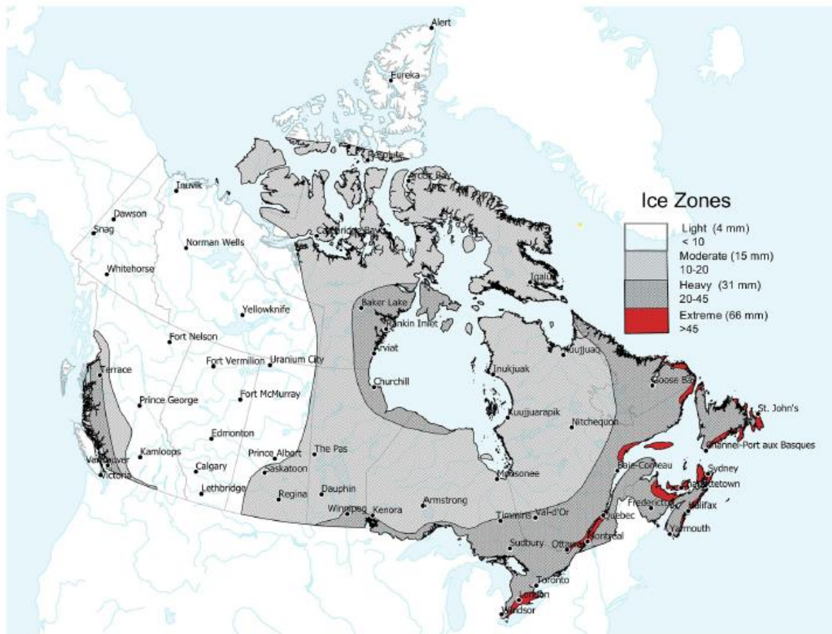
Figure 2-4: The nominal ice thickness zones and corresponding range (mm) (CSA S6, 2019).
