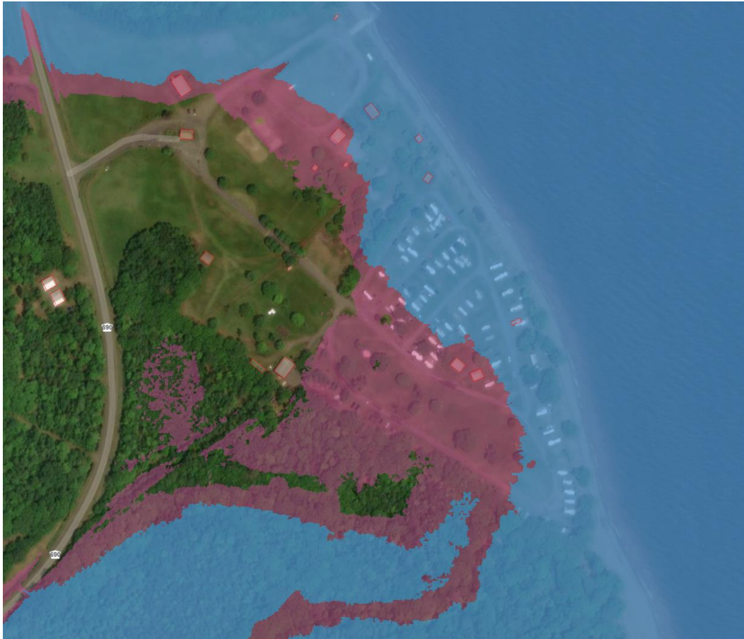
Figure 4-11 Princess Park Campground with flood zone overlay of 2018 floods (blue) and projected 100-year flood for 2100 (pink) (New Brunswick Flood Hazard Maps, n.d.).
