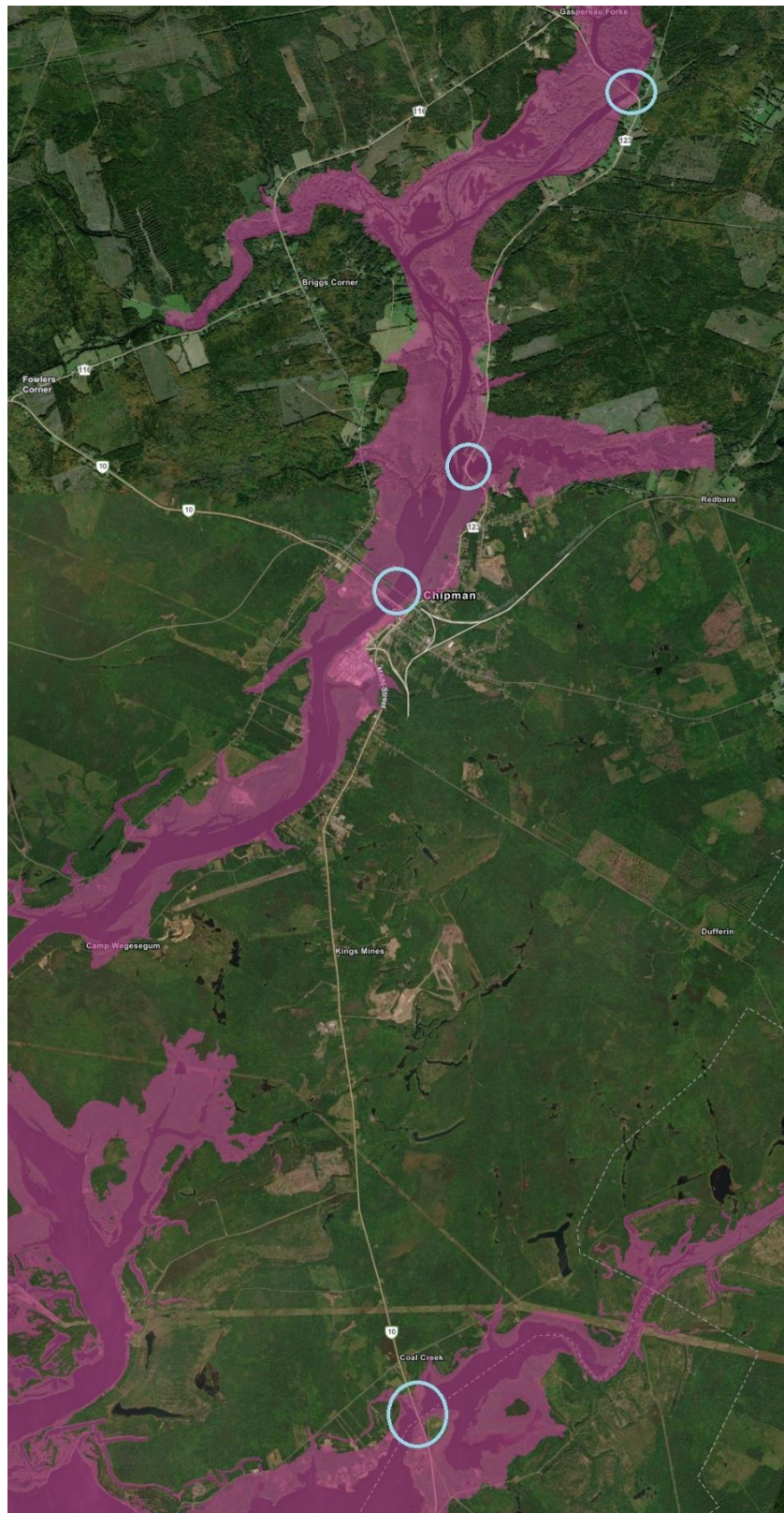
Figure 4-5 Map showing bridges providing access in and out of Chipman that will be inundated during 100-year flood event (New Brunswick Flood Hazard Maps, n.d.).
