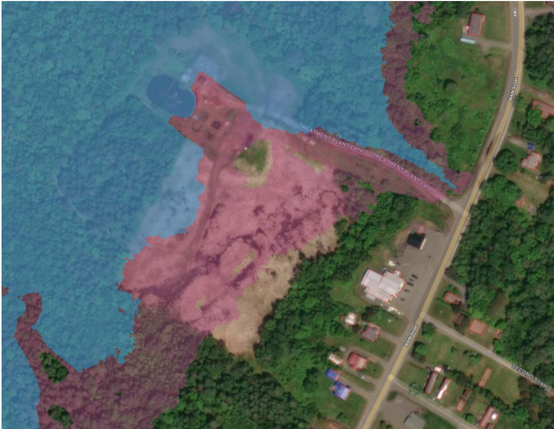
Figure 4-9 Chipman WWTP with flood zone overlay of the 2018 floods (blue) and the projected 100-year flood (pink) for 2100 (New Brunswick Flood Hazard Maps, n.d.).
