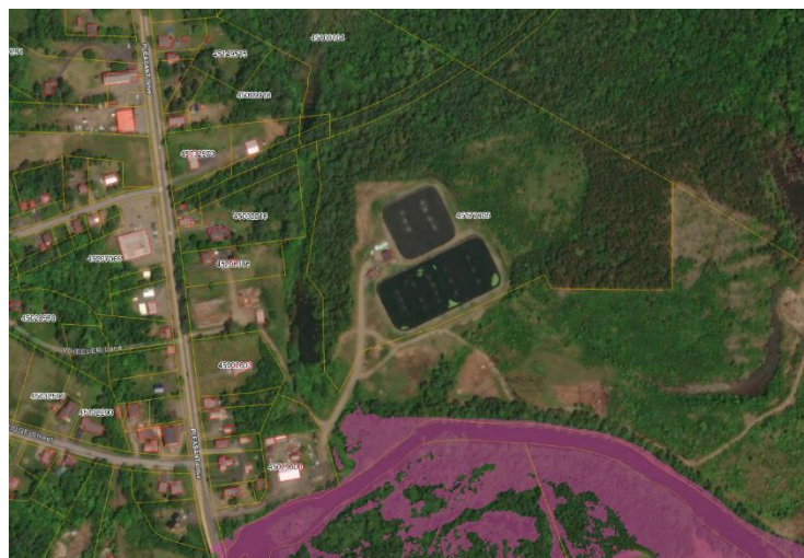
Figure 4-10 Minto WWTP with flood zone overlay of the projected 100-year flood for 2100 (New Brunswick Flood Hazard Maps, n.d.).
