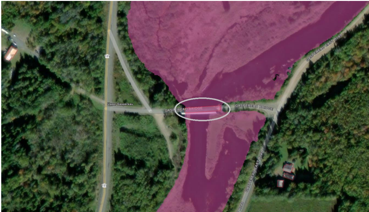
Figure 4-12 Burpee Bridge (Gaspereau Bridge) with flood plain overlay of the projected 100-year flood for 2100 (New Brunswick Flood Hazard Maps, n.d.).
